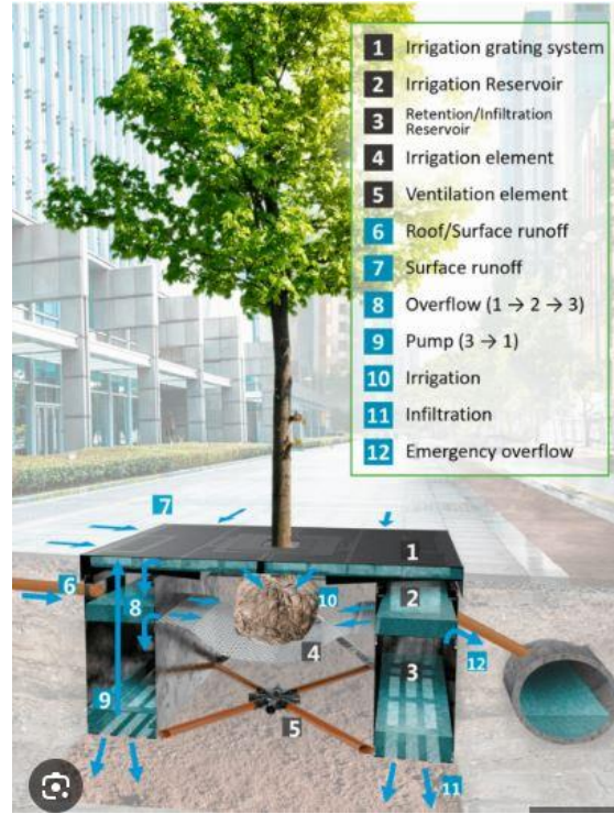
Мал. 3.9. Stormwater Tree Pits for Decentralized of Heavy Rainfall
