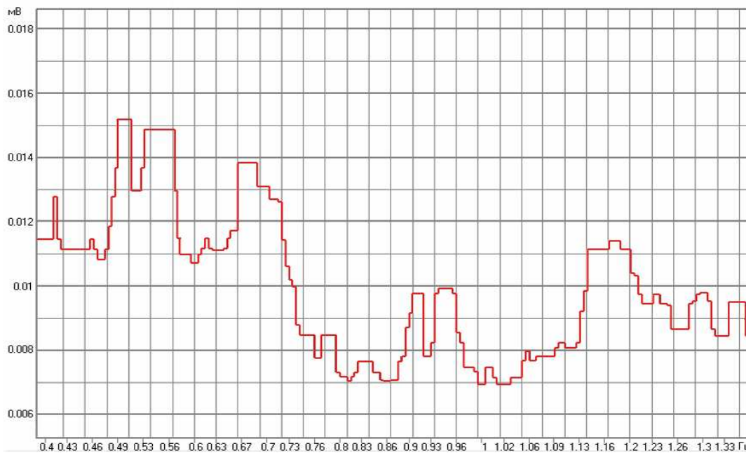
Fig. 2. The spectrum of natural vibrations of the IEC building
