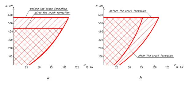
**Fig. 1.** The graphs of limits of the bearing capacity of the masonry pier before and after the crack formation at the central compression (according to SNiP II-22-81 [14]): a - of a vertical crack, b - of a horizontal crack
