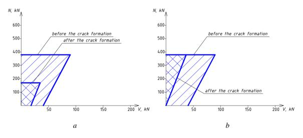
**Fig. 2.** The graphs of limits of the bearing capacity of the masonry pier before and after the crack formation at the eccentric compression (according to DBN V.2.6-162:2010 [15]): a - of a vertical crack, b - of a horizontal crack
