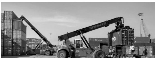
Figure 1. Use of reach stackers for handling operations with containers in cargo terminals and ports
