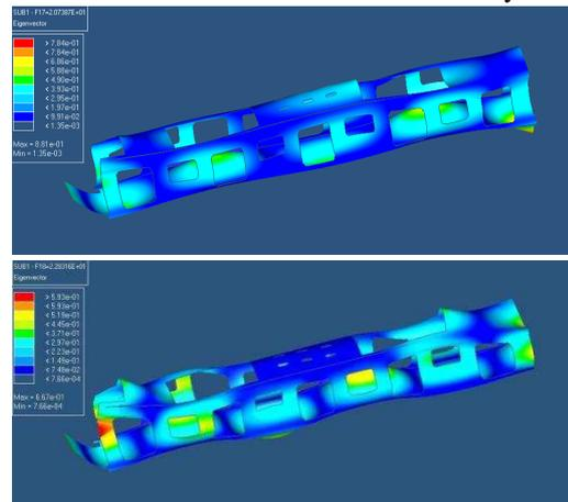
Figure 12 – The 17th and 18th vibration pattern of car body
