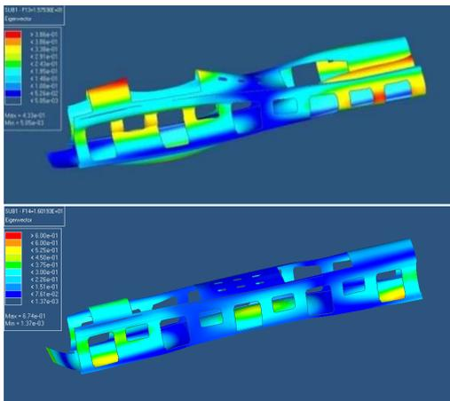
Figure 10 – The 13th and 14th vibration pattern of car body
