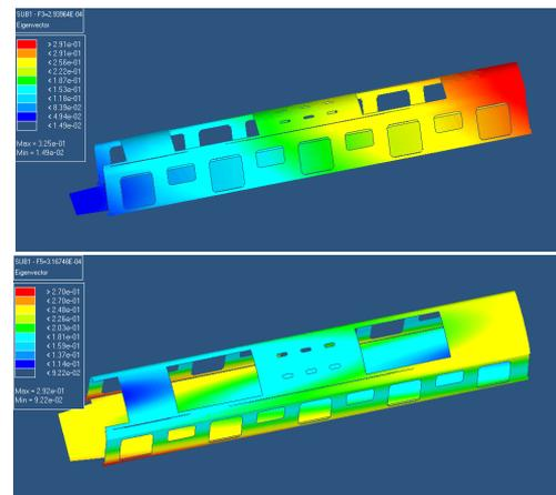
Figure 5 – Body 3rd and 4th vibration pattern
