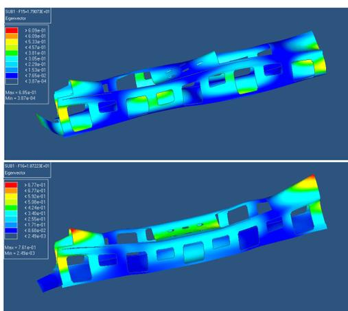
Figure 11 – The 15th and 16th vibration pattern of car body
