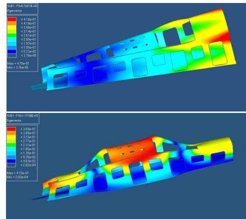
Figure 8 – The 9th and 10th vibration pattern of car body
