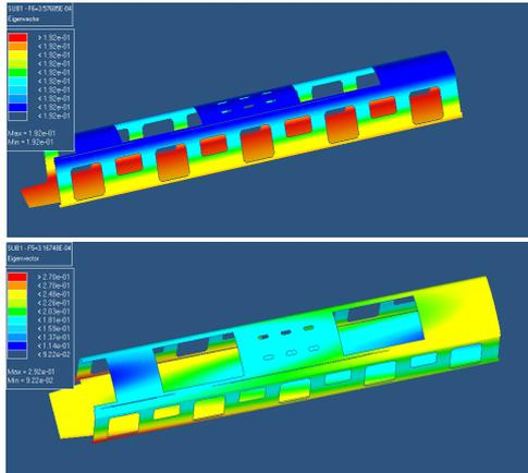
Figure 6 – The 5th and 6th vibration pattern of car body
