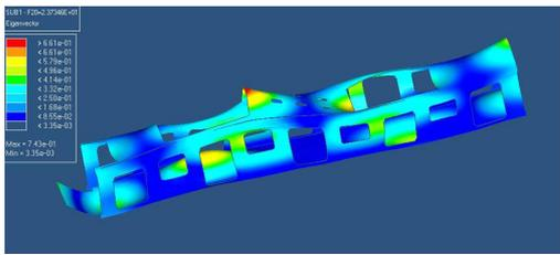
Figure 13 – The 19th and 20th vibration pattern of car body
