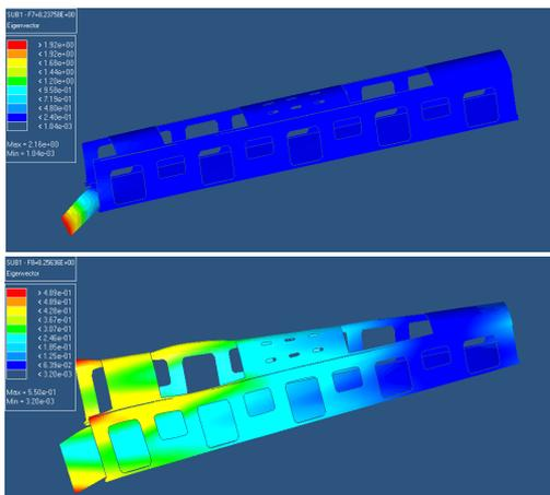
Figure 7 – The 7th and 8th vibration pattern of car body
