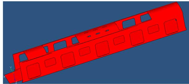
Figure 2 – Vehicle body model imported into HyperMesh
