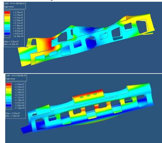
Figure 9 – The 11th and 12th vibration pattern of car body
