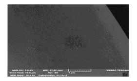
Fig. 7. The placement of active zones on the surface of basalt fiber
