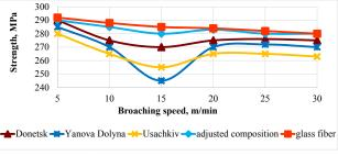
Fig. 6. The effect of melt cooling rate on the strength of basalt fiber
