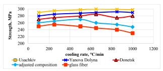
Fig. 5. The effect of the melt broaching speed on the strength of basalt fiber
