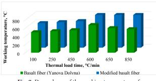
Fig. 9. Dependence of the working temperature of basalt fiber on the time of thermal load  $(T_{t.l.} - 1060 \text{ °C}, \emptyset 180-250 \text{ microns})$
