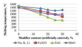
Fig. 4. The effect of modifiers on the melting temperature of the basalt charge
