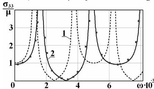
Fig. 2. Normalized stresses  $\sigma_{33}$  versus frequency  $\omega \cdot 10^{-3}$
