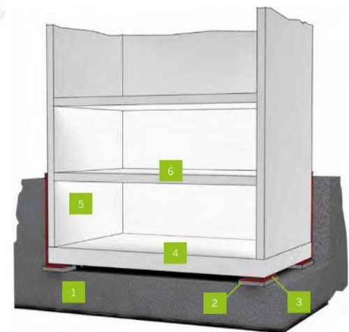
Point decoupling of a building foundation with Regupol®/ Regufoam® vibration damping material: 1 natural surface • 2 impedance plate • 3 Regupol®/ Regufoam® vibration isolation • 4 foundation plate • 5 basement wall • 6 floor slab
