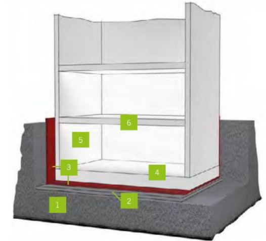
Full-surface decoupling of a building foundation with Regupol®/ Regufoam® vibration damping material: 1 natural surface • 2 impedance plate • 3 Regupol®/ Regufoam® vibration isolation • 4 foundation plate • 5 basement wall • 6 floor slab
