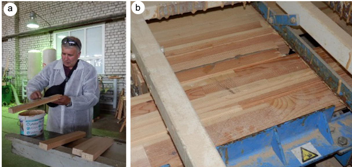
Fig. 1. Application of the glue to wood ladders (a) and following curing under pressure (hydraulic press of the company R. Beck Maschinenbau, Germany) (b)
