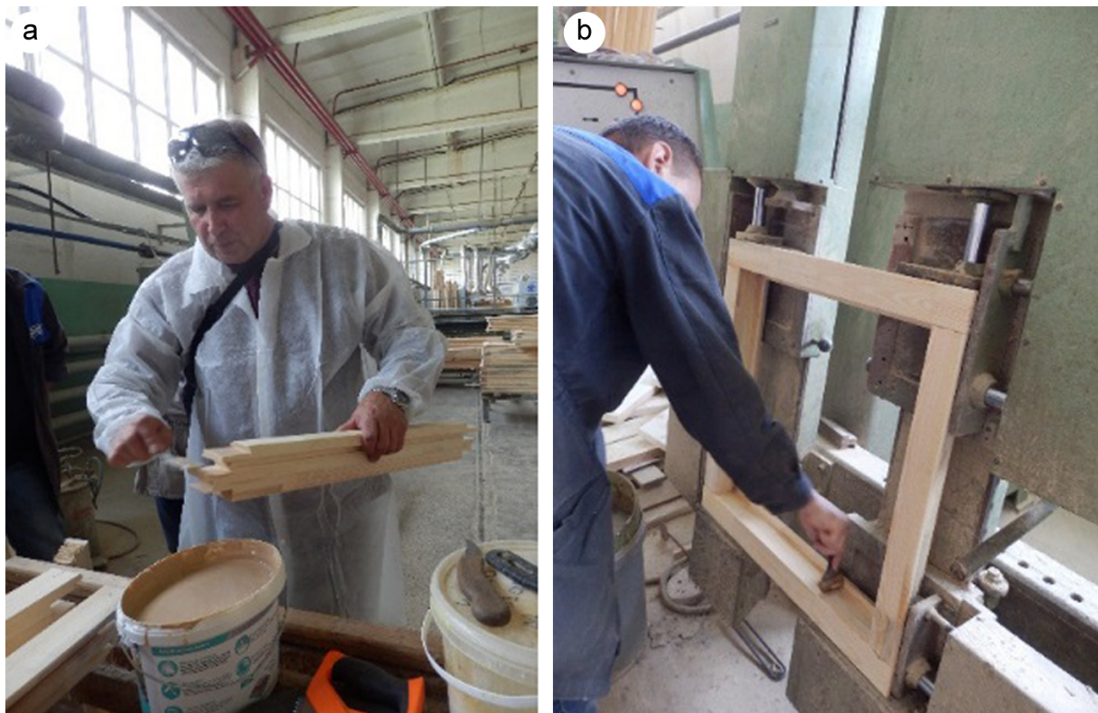
Fig.2. Application of the glue to the corner dowelled connections of a window frame (a) and following pressing (a hydraulic press of the company Waima, Germany) (b)
