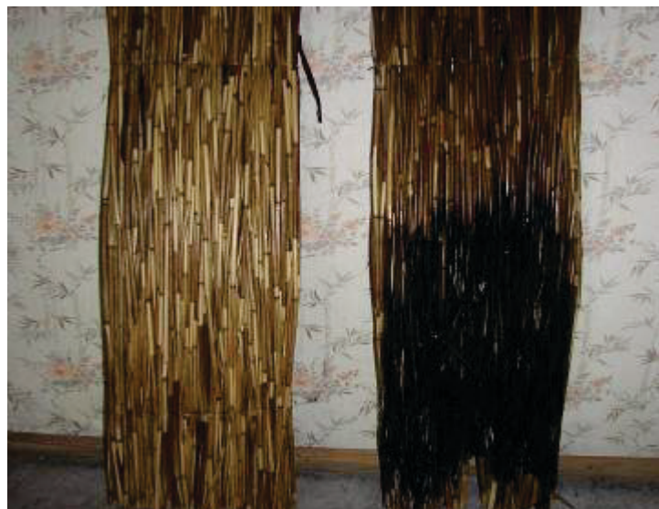
Figure 5. Results of determining the flammability of a fire retardant cane sample.
