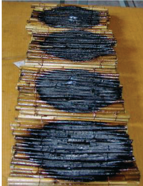
Figure 3. Appearance of cane beams treated with a protective composition after the influence of the heat flux during the determination of flammability.
