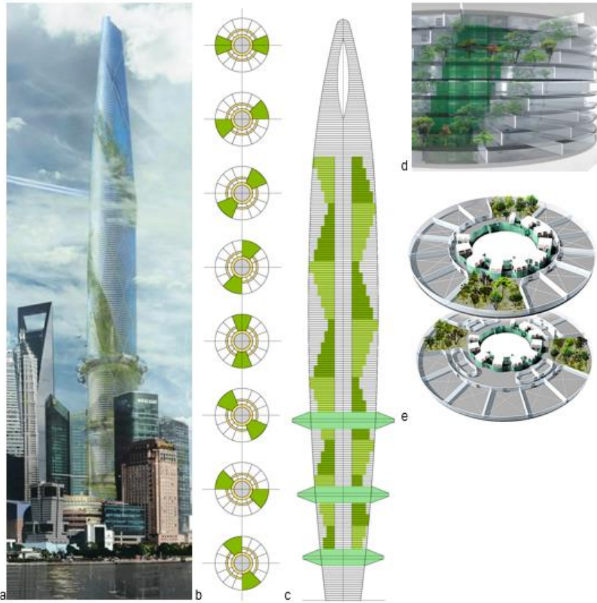
Figure 5 A three-dimensional planning solution of the biotecton planting system: a – general view of "Biotecton", b – floors with greening; c – section of greening; d – general view of "green zones"; e – turn of greening zones on different floors
