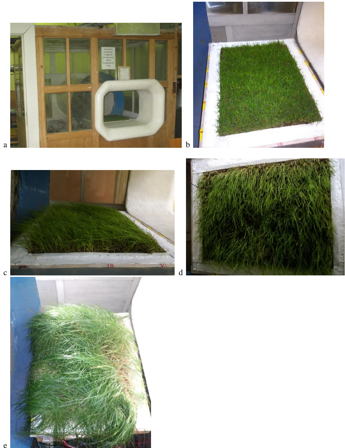
Fig. 1. Experiments of cooling effect in wind tunnel: a – the wind tunnel with the model; b – the grass with high 40 mm; c – the grass with high 123 mm; d – the same, top view; e – the grass with high 399 mm
