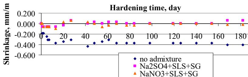
Fig. 1. Development of proper deformations in alkali-activated portland cement modified with complex admixtures
