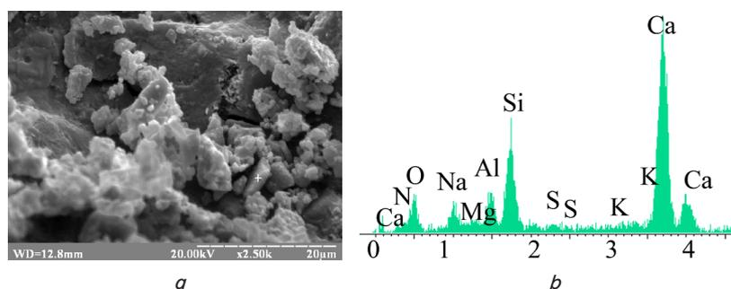
Fig. 8. Characteristics of microstructure of alkali-activated slag cement modified with complex admixture “clinker–NaNO<sub>3</sub>–SLS–SG” after 28 days of strengthening: *a* – electron micrograph of the cleavage surface; *b* – probe analysis
