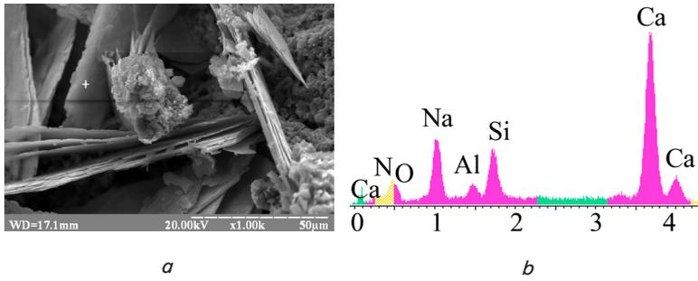
Fig. 5. Characteristics of microstructure of alkali-activated portland cement modified with complex admixture “NaNO<sub>3</sub>–SLS–SG” after 28 days of hardening: *a* – electron photomicrograph of the cleavage surface; *b* – probe analysis
