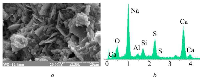
Fig. 4. Characteristics of microstructure of alkali-activated portland cement modified with complex admixture “Na<sub>2</sub>SO<sub>4</sub>–SLS–SG” after 28 days of hardening: *a* – electron photomicrograph of the cleavage surface; *b* – probe analysis
