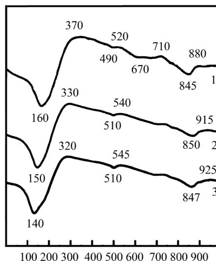
Fig. 2. Curves of differential-thermal analysis of AAPC (on day 28 of hardening): 1 – with no admixture; 2 – with complex admixture “Na<sub>2</sub>SO<sub>4</sub>–SLS–SG”; 3 – with complex admixture “NaNO<sub>3</sub>–SLS–SG”
