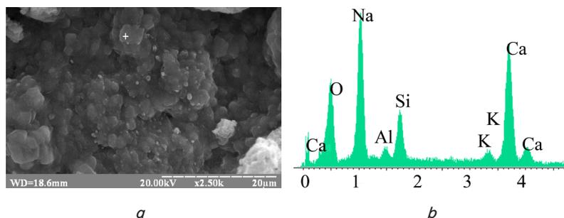
Fig. 3. Characteristics of microstructure of alkali-activated portland cement after 28 days of hardening: *a* – electron photomicrograph of cleavage surface; *b* – probe analysis
