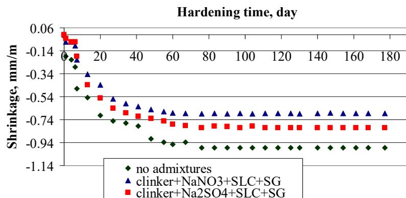
Fig. 6. Development of proper deformations in alkali-activated slag cement when using complex admixtures of “clinker–salt electrolyte–surfactant” system
