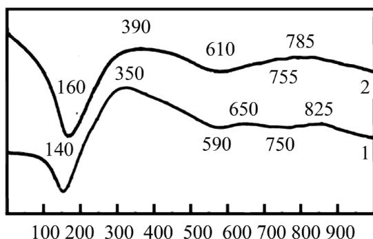
Fig. 7. Curves of differential thermal analysis (on day 28 of hardening) of alkali-activated slag cement: 1 – with no admixtures; 2 – with complex admixture “clinker–NaNO<sub>3</sub>–SLS–SG”
