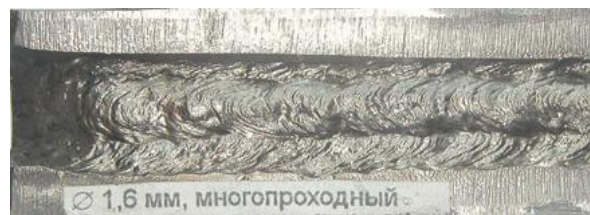
Fig.4. Formation of metal of multilayer weld
