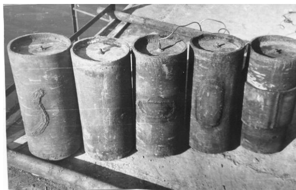
Fig.7. The samples simulating repair of the typical defects of pipelines after testing under inner pressure of 5 MPa
