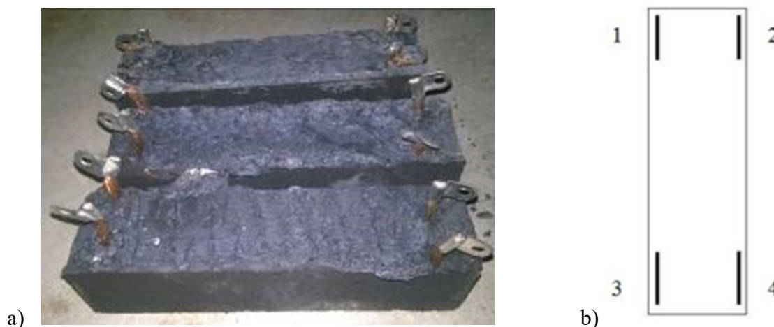
Fig. 1. Experimental samples from electroconductive concrete: a) samples; b) layout of electrodes
